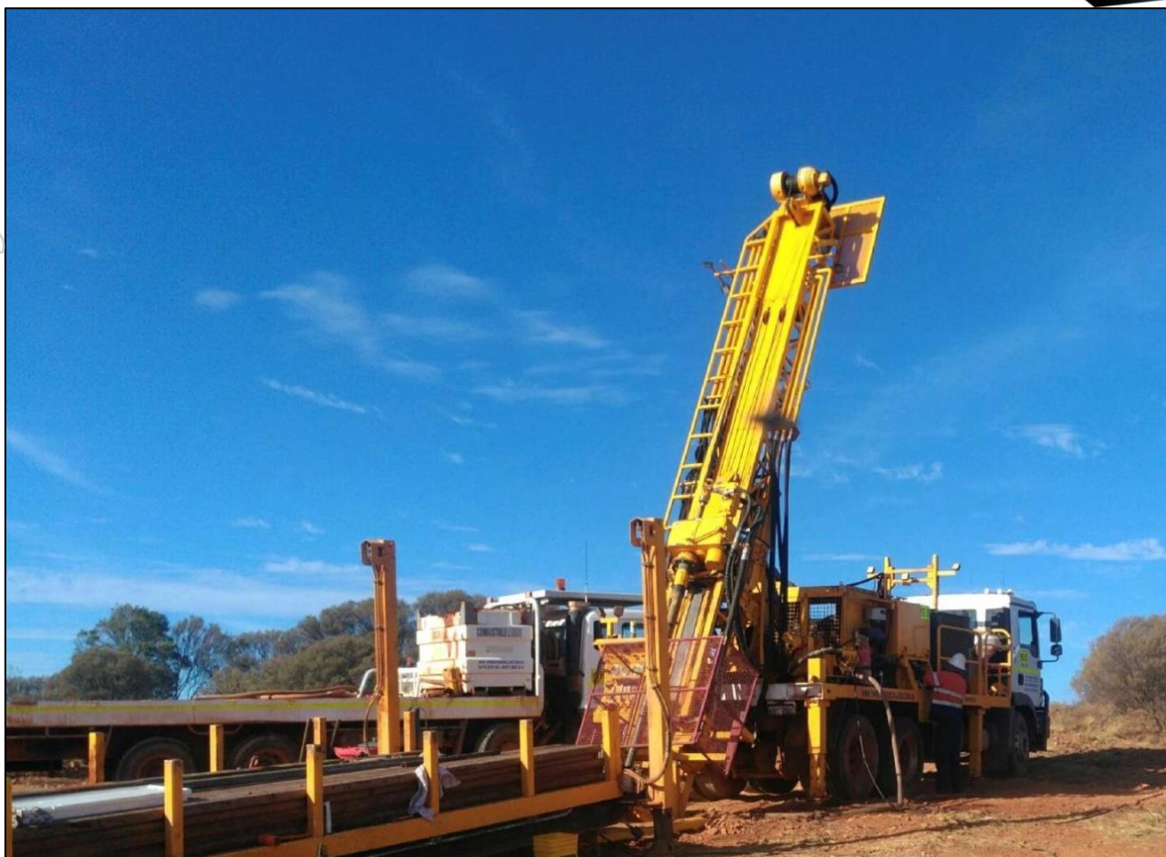
Image 1. Diamond Core Drill Rig operating at the Earahedy Project
